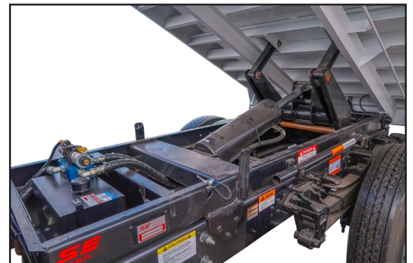
Dual manual-control Hoist Secure Locking Arms
